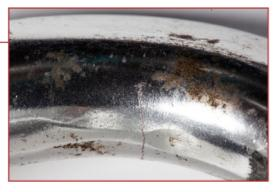
Initial surface cracks within the karabiner attached to the TRAC or TRAC plus pulley may go unnoticed as they form in the area of contact and are generally out of sight. (See below). Affected karabiners should be identified and removed.
